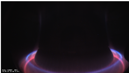
Figure 1: Visible camera image of a discharge with an XPR (AUG #40007, 3.4s) seen in blue light emitted by nitrogen, dominated by N^{2+} . Magenta is the typical Balmer emission from deuterium in a divertor leg.
