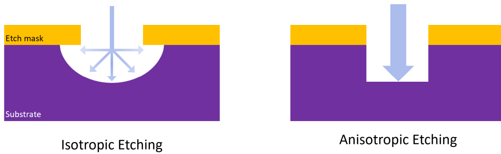
Figure 1-14 Two categories of etching directionality. (a) Shows the isotropic etching where the reaction occurs in multiple directions within the substrate leading to an undercut. (b) Shows an anisotropic etching that is highly directional and can make straight walls in the substrate.
