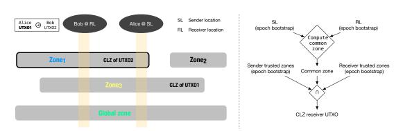
Figure 3.6: Nyle's choice of CLZ. The output  $UTXO_2$  is assigned as CLZ Zone<sub>1</sub>, which is the common trusted zone of Alice and Bob with the smallest exposure. The CLZ is uniquely determined by participant values provided in the beginning of each epoch.
