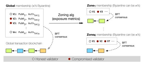
Figure 3.3: Nyle secure zoning. Nodes join the Global zone membership and claim a provable location. Based on these claims, anyone can obtain the local zones' memberships by running the zoning algorithm. The Global zone is secure, but local zones can be compromised.
