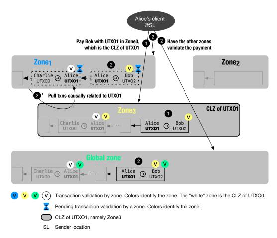
Figure 3.5: Transaction validation in Nyle. Alice sends  $UTXO_1$  to Bob. (1) Alice submits the txn for validation to Zone<sub>3</sub>, which is the CLZ of  $UTXO_1$ . (2) Alice submits the txn to other zones that overlap her location. The CLZ Zone<sub>3</sub> acts as a single point of synchronization for  $UTXO_1$ , assisting to prevent double-spending.
