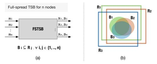
Figure 4.2: Full-spread TSB (FSTSB). (a) FSTSB is a group communication primitive, where each node inputs a message and outputs two sets *R* (received messages) and *B* (messages received by other nodes). The respective sets of different nodes may not be the same. The guarantee is that  $B_i \subseteq R_J \forall I, J, K \in \{1, ..., n\}$ . (b) Illustrative example of the *R* and *B* set relationship for three nodes.
