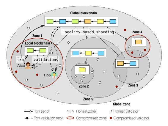
Figure 3.2: Final Nyle design using a trust-but-verify principle. Multiple zones independently validate each transaction, and the sender/receiver can choose which validations to wait for. Local zones limit Lamport exposure but might be malicious, whereas the Global zone always acts as the possibly slow but secure transaction finalizer.
