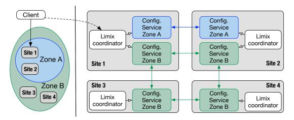
Figure 2.5: Limix's architecture on a simplified example with four sites and two zones.
