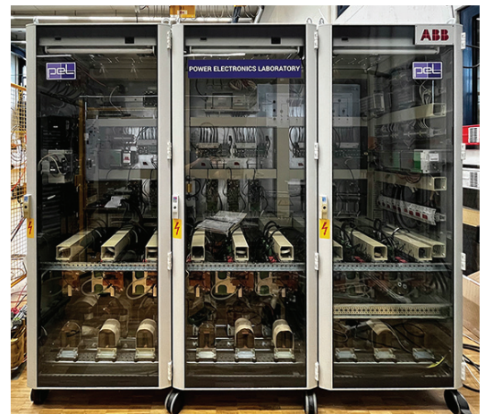
Fig. 5: The LV PETT prototype, which serves as SST research platform for the works presented in this paper.
