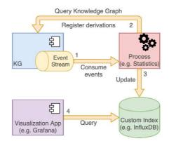
Fig. 10. Clients and services can subscribe to the event log stream, query the knowledge graph for additional information, generate derivations to be registered back into the system or maintain third-party indices.
