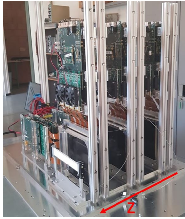
FIGURE 8: The SciFi tracker setup, with the boards separated spatially in the z direction [3].
