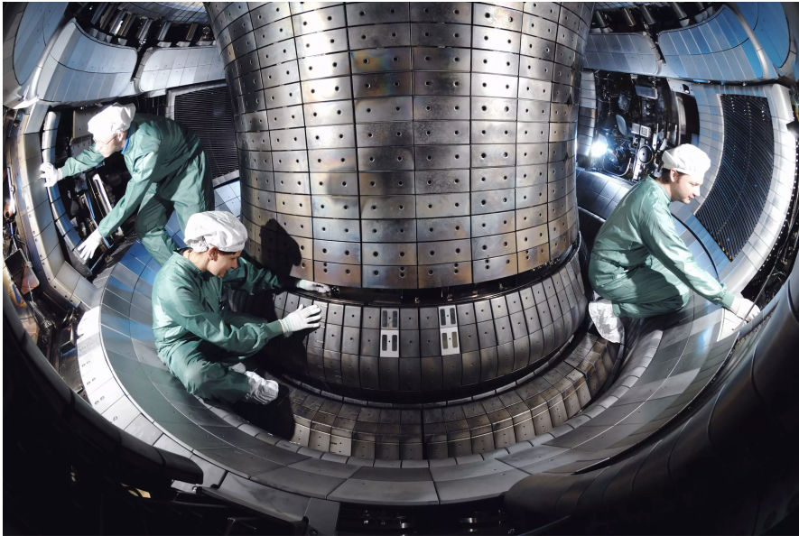
Figure 1.6: Inside the AUG vacuum vessel, note the tungsten tiles. Source: www.ipp.mpg.de .
