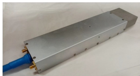
Fig. 6: Engineering Model of Ku-band Dual Mini-TWT. The mass of the dual-TWT (without cable) is under a kg.
