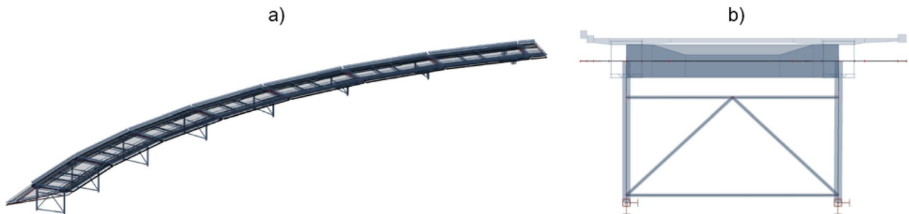
Fig. 2 Finite-element model of the bridge. (a) Overview of the model; (b) cross-section
