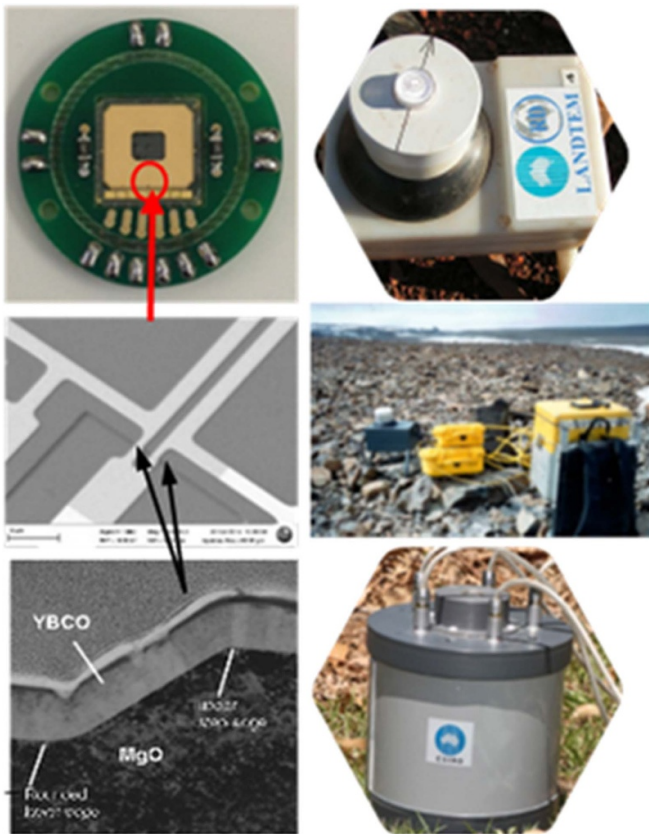
Figure 13. CSIRO HTS SQUID left: an 8 mm pickup-loop dc SQUID magnetometer with close views of the SQUID loop and a TEM image [96] of a step-edge junction and SQUID instruments (right: LANDTEM mineral exploration tool [98] and UXOMAG magnetic tensor gradiometer for MAD) operating in a rugged hostile environment. Reproduced from [96]. © IOP Publishing Ltd. All rights reserved. Adapted from [98], with permission from Springer Nature. Reproduced from [99]. © IOP Publishing Ltd. All rights reserved.
