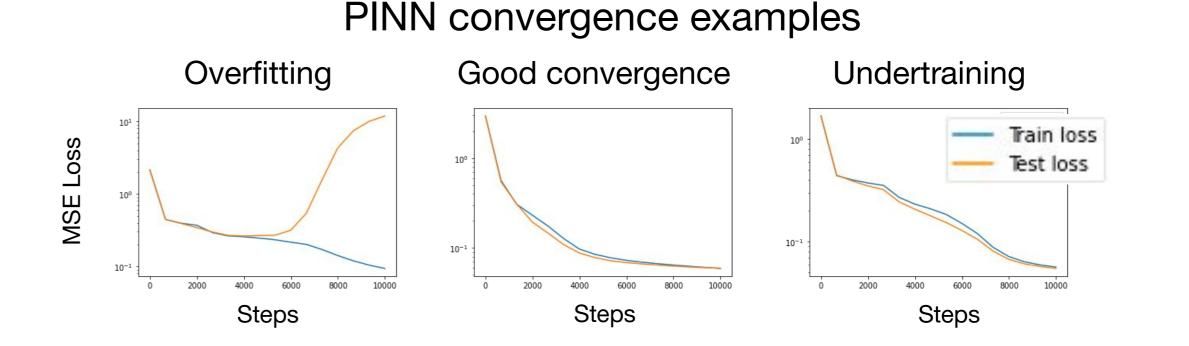
The DNN with the addition of the PINN output performs largely the same as the original geometric DNN from [2]. However, our models have significantly smaller distances between train and test curves.
