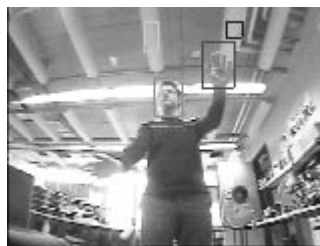
Figure 27: No gesture could be extracted because hand has no skin color (due to saturation effects around the hand)
