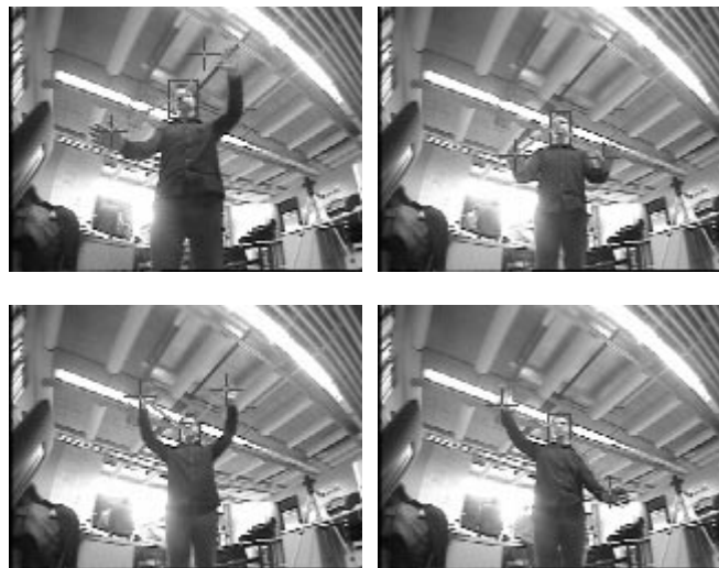
Figure 26: Successful gesture extraction: go back, follow me, stop, go forward (from top left to bottom right)
