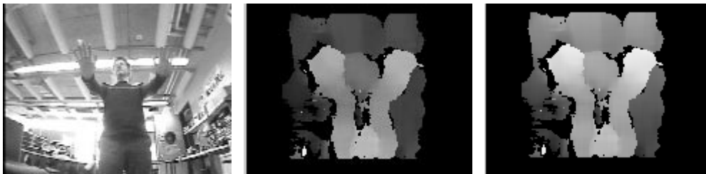
Figure 8: Original image (left), disparity map unprocessed (middle) and processed (right) to correct disparity
