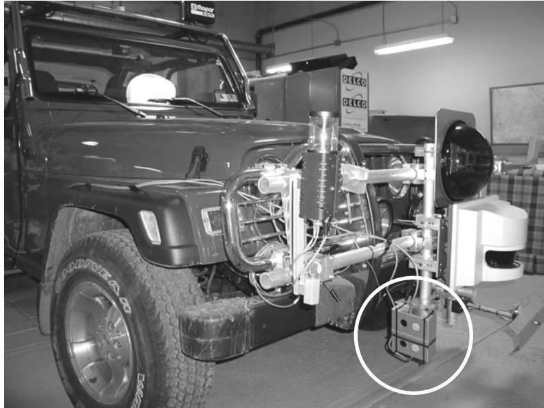
Figure 34: The curb detection setup. Two sensors are mounted next to the front bumper (in the center of the white circle)
