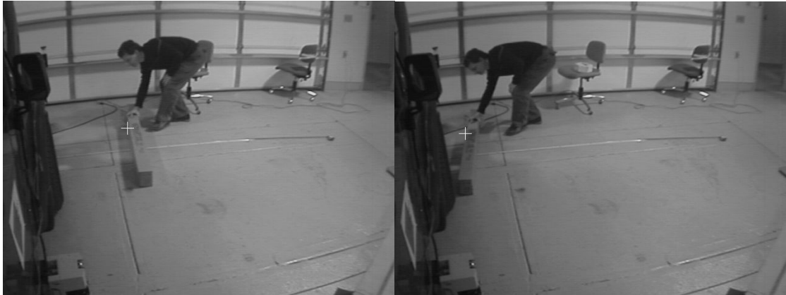
Figure 35: Detection of the curb in the lab at several distances. The white cross designates where the system sees the curb.
