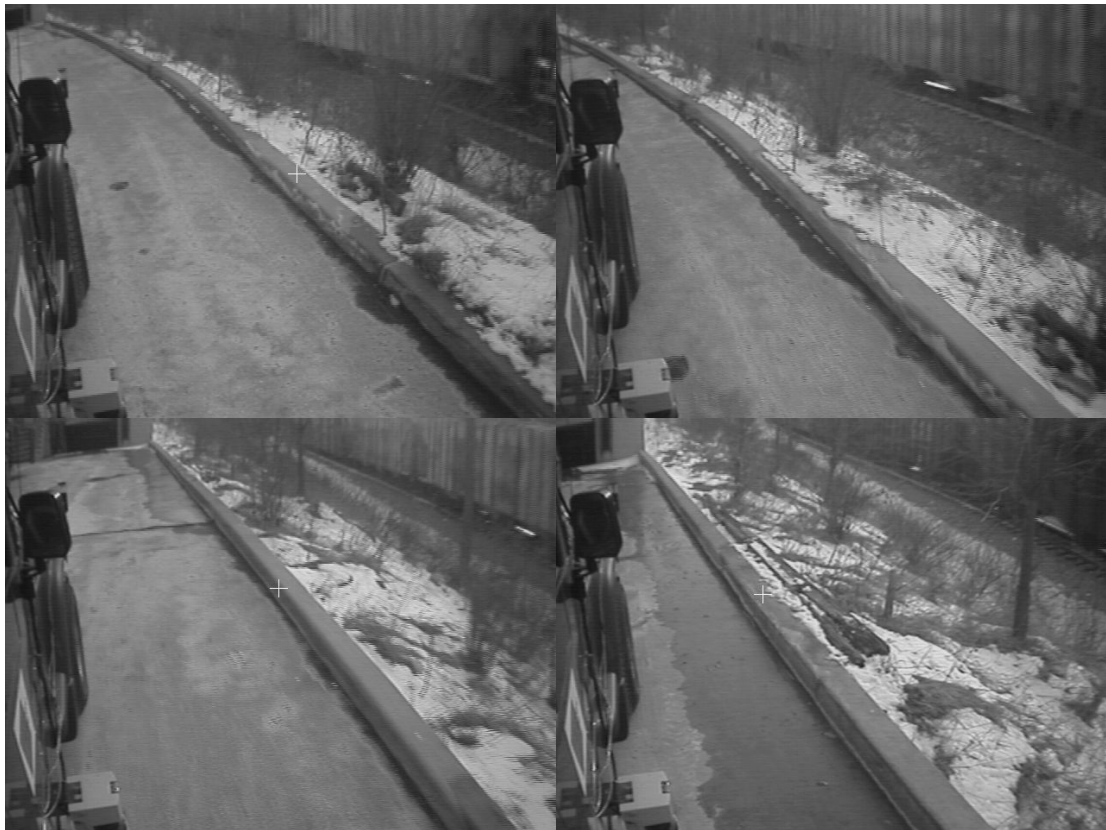
Figure 36: Detection of the curb on the CMU campus. On the top right image, detection failed
