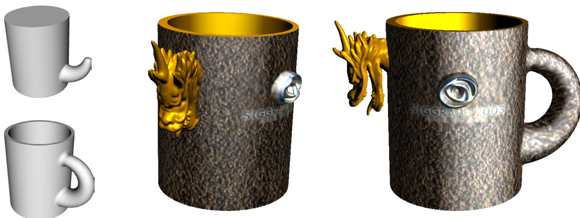
Figure 8.6 Creating a coffee mug using boolean operations, deformation, collision detection and particle-based blending.
