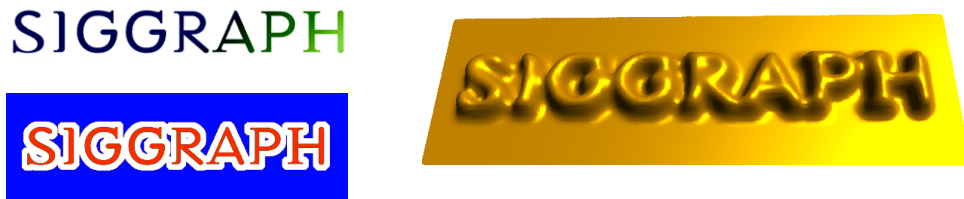
Figure 6.13 Embossing effect. The Siggraph label on the top left has been converted to a selection stencil using simple image processing tools. This stencil can then be mapped to a surface, where blue color corresponds to the zero-region and red to the one-region. Subsequent deformation yields an embossing effect as shown on the right.
