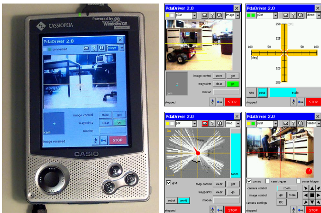
Figure 1. PdaDriver and control modes: image ( top center ), direct ( top right ), map ( bottom center ), sensor ( bottom right )
