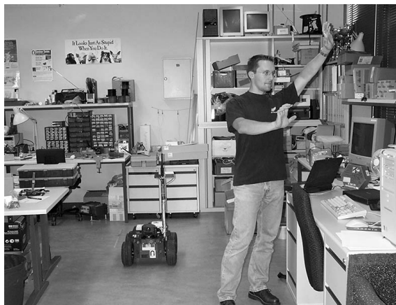
Figure 7: Visual gesturing for vehicle teleoperation
