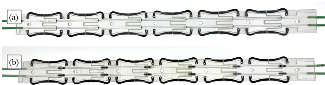
Figure 5.27: Array of samples with the spring-based solution. (a) Face seal and (b) radial seal hydraulic interfaces.
