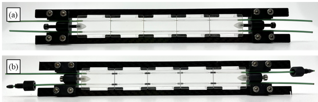
Figure 5.29: Samples array of the rail-based solution. (a) Face seal and (b) radial seal hydraulic interconnections. Note that only one pusher is sufficient to compress the micro O-rings (b).
