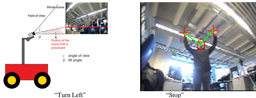
Fig. 6. Robot configuration and static gesture recognition for robot motion control
