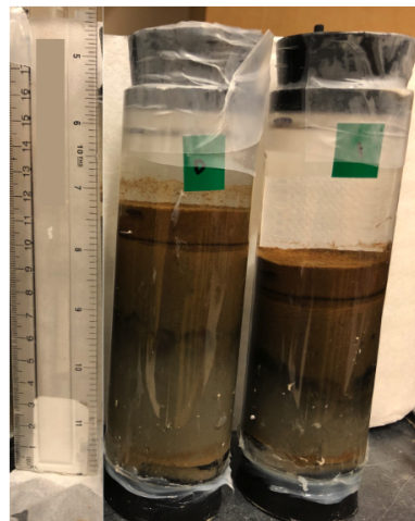
Figure S6. Photos of cores used in incubation experiments at a. 0.1 - 0.2 % atmospheric oxygen, b. 5.5 - 5.7 % atmospheric oxygen, and c. 21 % atmospheric oxygen. The top layer of slightly darker sediment material was less consolidated than layers below and moved with overlaying water.
