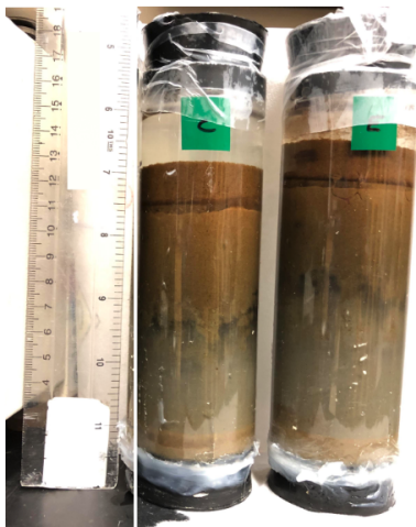
Figure S6. Photos of cores used in incubation experiments at a. 0.1 - 0.2 % atmospheric oxygen, b. 5.5 - 5.7 % atmospheric oxygen, and c. 21 % atmospheric oxygen. The top layer of slightly darker sediment material was less consolidated than layers below and moved with overlaying water.
