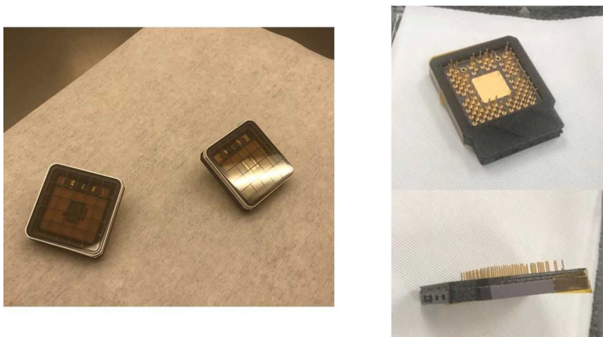
Figure 7.5: AMCP chips integrated into a Planacon tube, front (left) and backside (right).
