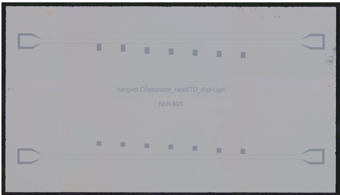
Figure C.5 | Hanged resonators. 7 \times 4 mm 2 chip with the test structures resonators used for film characterization. The two feedlines are coupled to either seven 500 nm wide resonators or 250 nm wide resonators in hanged configuration. The specific chip was design to impedance match films with an expected kinetic inductance of 60 pH.
