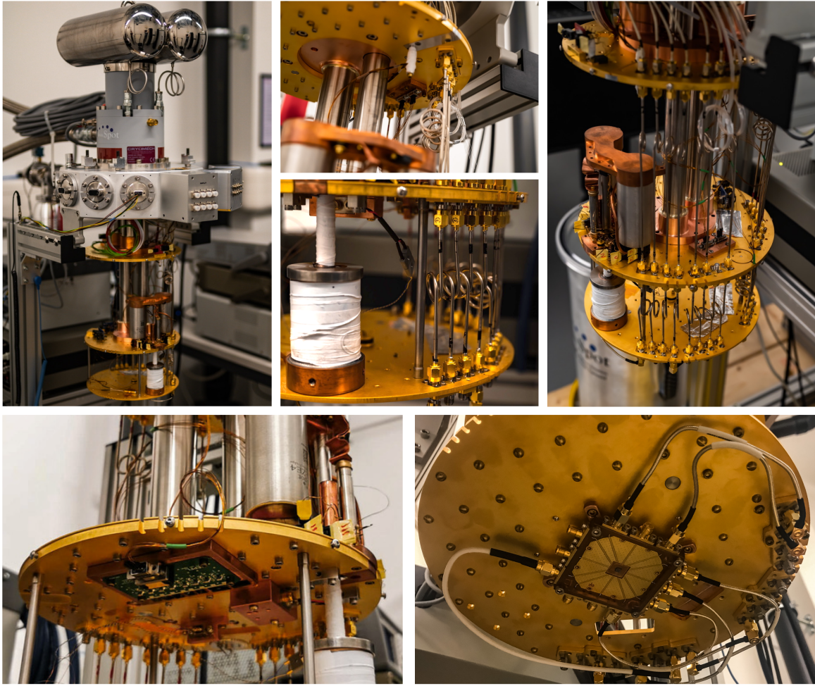
Figure B.1 | PhotonSpot cryostat. The cryogenic systems within the PhotonSpot consist of a pulse tube cryocooler, to bring the system down to 3 K, and a ^4\text{He} sorption cryocooler, to cool the cold plate down to 800 mK. The advantages of such a system is the time of cooldown, which is in the order of 2h to reach 3 K and 12h to reach base temperature, and the advantage that being a closed-loop system there is no consumption of cryogens required.
