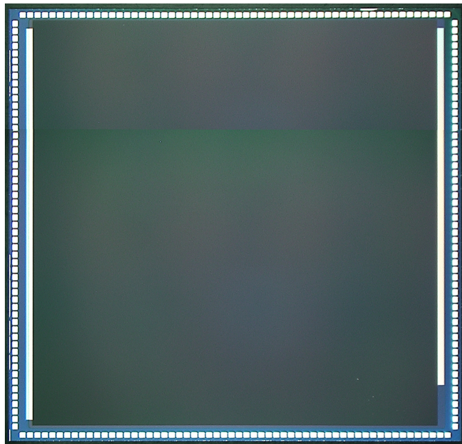
MegaPhase (Chapter 3). Die size is 8 \times 7.5 \text{ mm}^2 .
