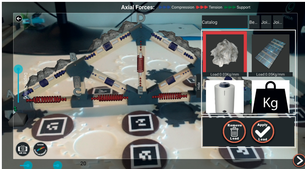
Figure 7-8 · Adding statics information on the beams
