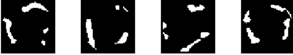
Figure 4.12: Selected cross-sectional bubble hold-up reconstructions from a measurement height of 6 cm that are likely the result of limited measurement angles.
