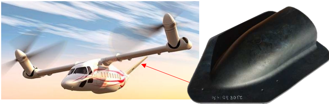
Figure 12. Leonardo's NGCTR Technology Demonstrator with rTPC Fairing (modified from [13])
