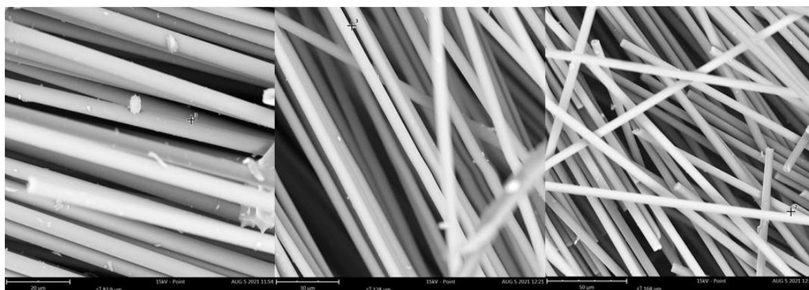
Figure 6. SEM images of the carbon fibers after oxidation at 450°C (left), 500°C (centre), 550°C (right).
