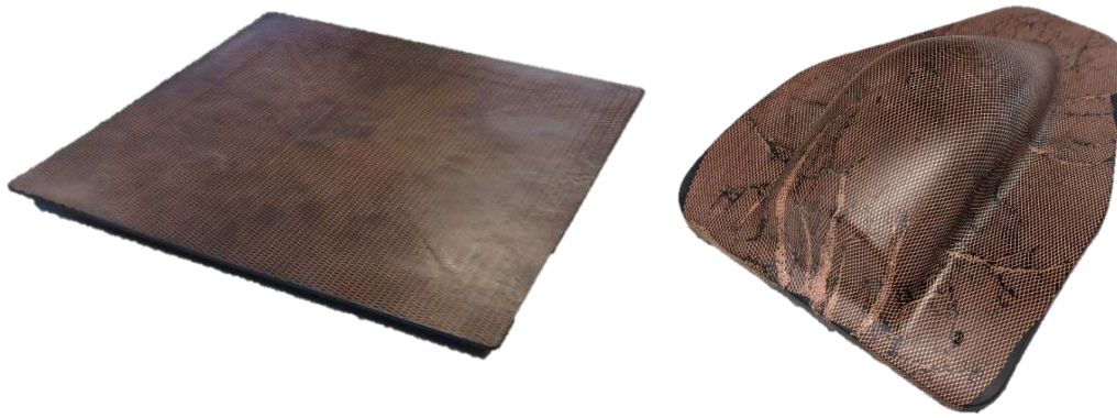
Figure 9. Typical Results for Integrated LSP Foils on Flat and Contoured Parts
