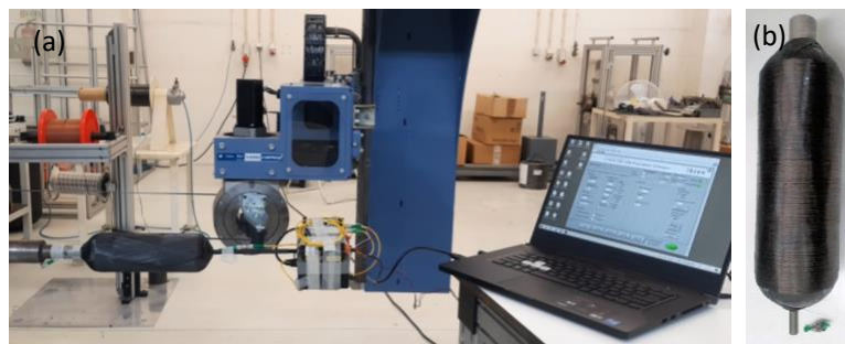
Figure 2: Production of the COPV by tape winding
