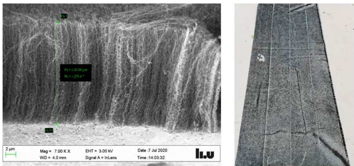
Figure 1 : (Left) VACNT forest on stainless steel substrate. (Right) VACNT forest deposited on prepreg surface.
