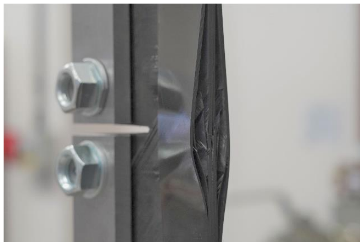
b) Test 1 specimen showing compressive failure at the rear without stringer failure. Stringers at the rear of the specimen have bulged out due to compression, no stringer cracking observed.
