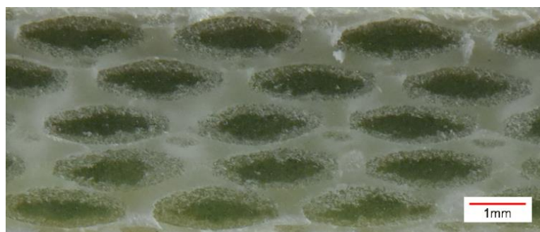
Figure 5: Picture of the cross-section of a PP plate pressed at 10.4 bar for 5 minutes.
