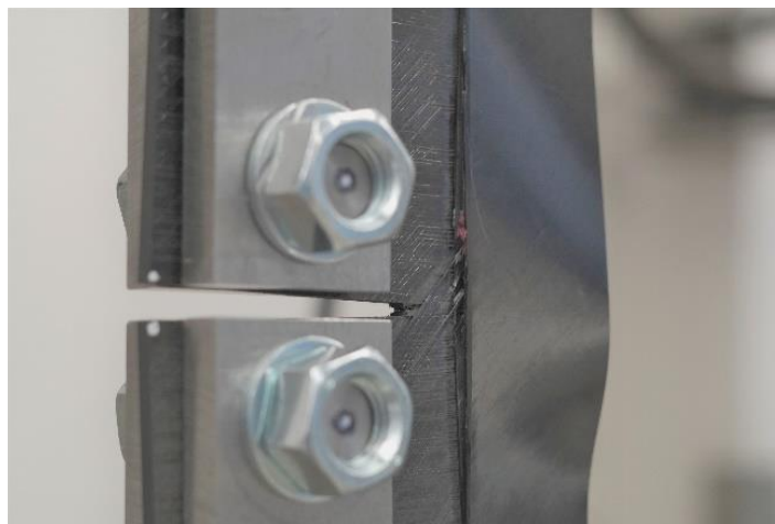
a) Test 1 after compressive failure showing large area of skin-stringer debonding without stringer failure.
