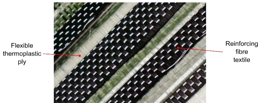
Figure 1: Picture of a partial cutaway of quasi-UD carbon / PEI hybrid textile manufactured at the Faserinstitut Bremen.
