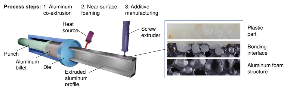
Figure 1. Schematic illustration of a manufacturing process for hybrid structures
