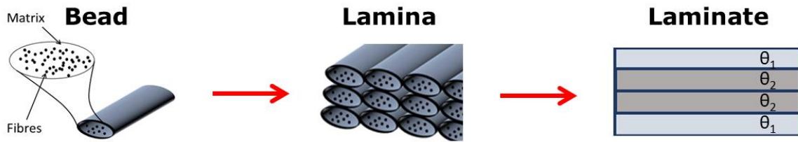
Figure 1 Manufacturing process of 3D-printed composite laminates with various orientations \vartheta .
