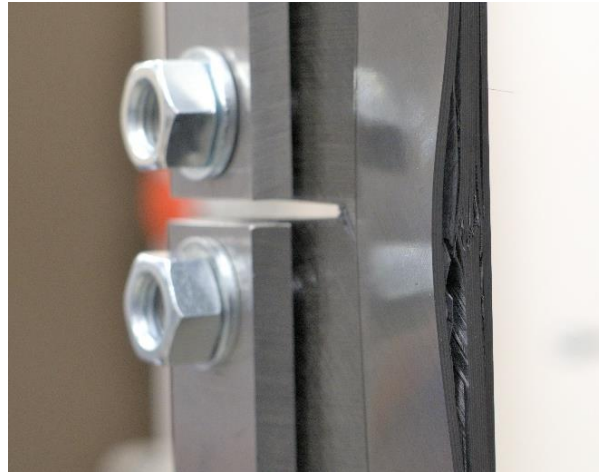
b) Test 3 specimen showing skin compressive failure at the rear and skin-stringer debonding.
