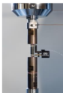
Figure 1. Set-up of cyclic tensile tests.
