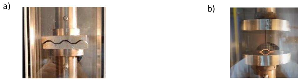
Figure 2. Thermoforming set-up mounted on a tensile machine; a) 1 st Thermoforming set-up of zigzag mould. b) 2 nd Thermoforming set-up of flat compression plates
