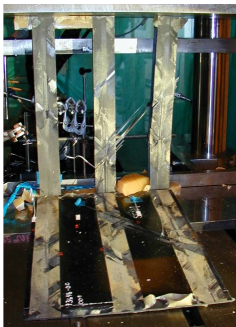
Figure 8. Multiple stiffeners debonding from a panel under compression [1] (courtesy of Ministry of Defence)
