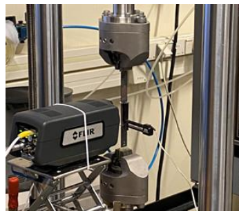
Figure 2. FLIR A6752sc thermal imaging camera positioned to measure self-heating during cyclic mechanical loading
