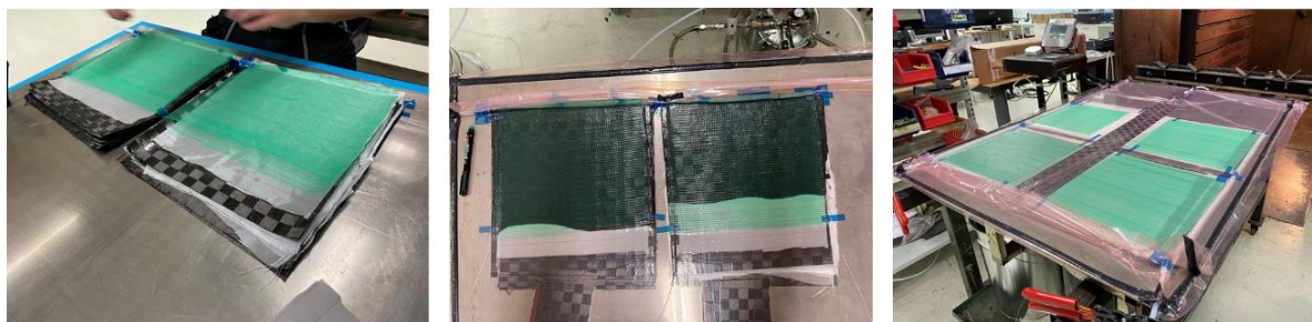
Figure 1. Manufacturing of hybrid thin-ply laminates with vacuum infusion
