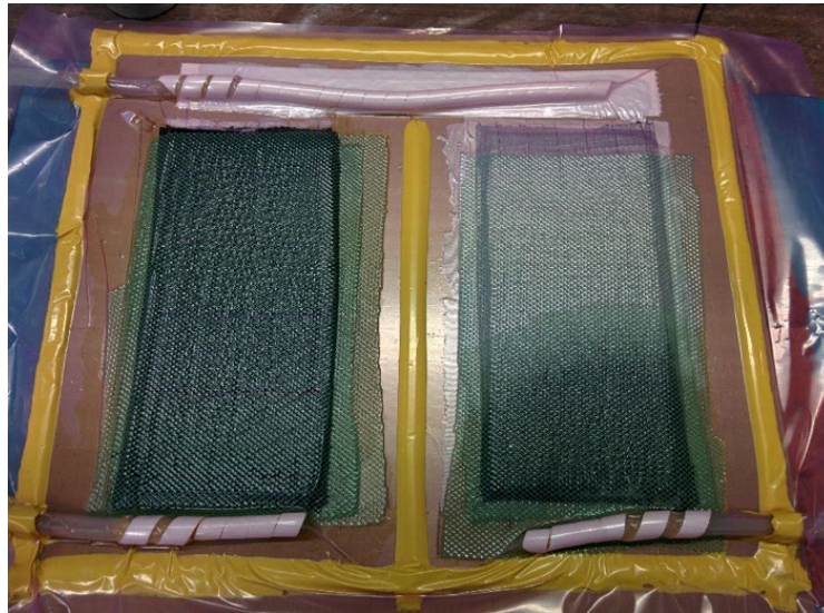
Figure 2. Vacuum assisted resin infusion molding.
