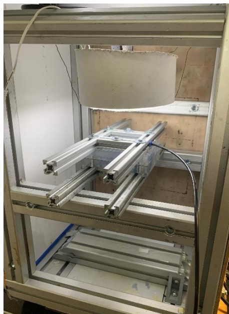
Figure 2: Test rig for the optical analysis of the impregnation
