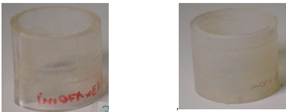
Figure 8: Degraded silicone covers: Sylgard 184 after 170 m (left) & SF45 after 450 m (right)
