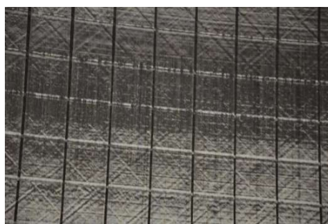
Figure 1 : Grooved laminate due to insufficient gap sizes placed with in-situ T-AFP
