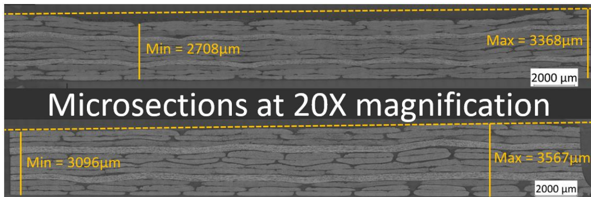
Figure 10. Microsections of compaction barrier region. Top) No relaxation Bottom) 5-minute relaxation cycle
