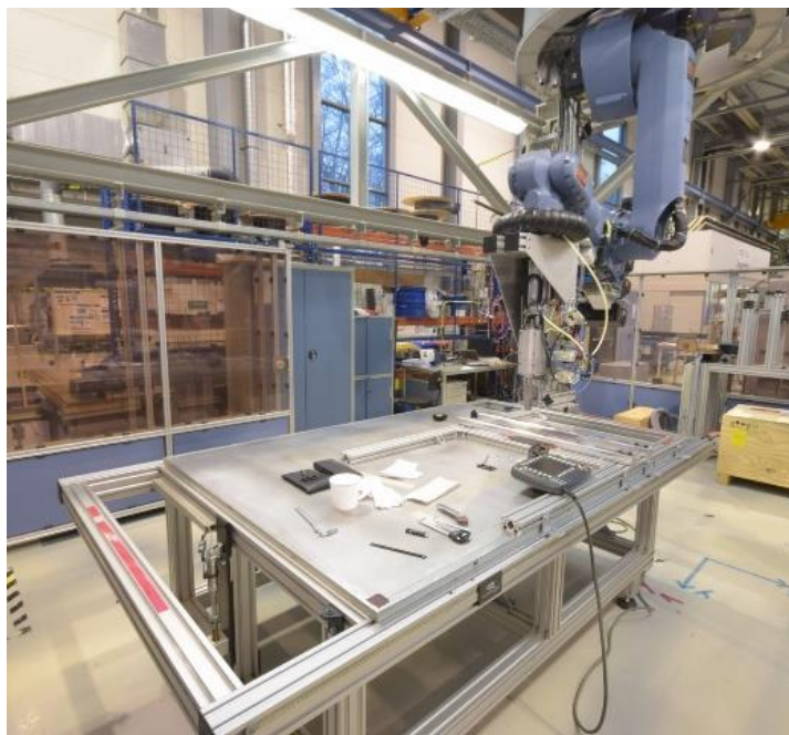
Figure 1. Robotic ultrasonic welding cell at CTC GmbH in Stade
