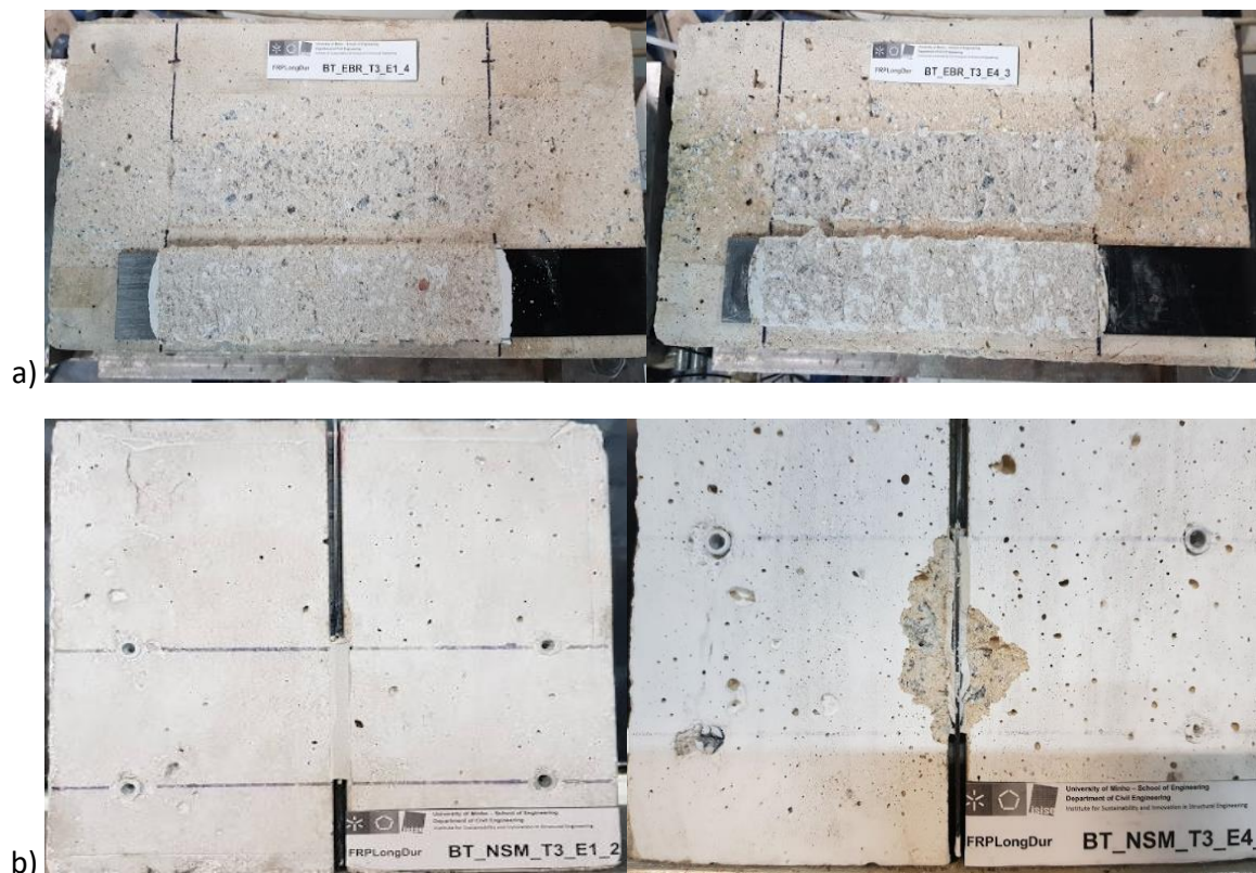
Figure 6. Typical failure modes observed after three years of exposure: (a) EBR specimens, (b) NSM specimens
