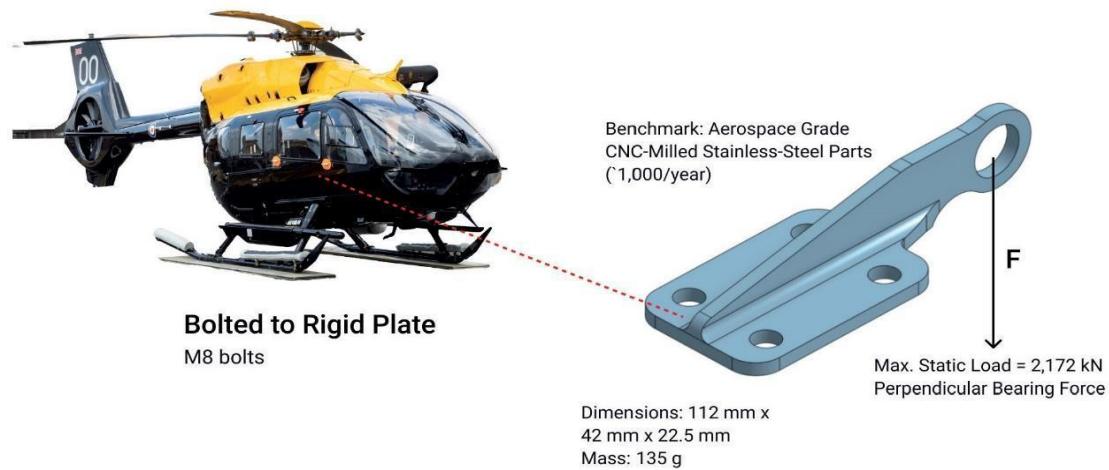
Figure 3: Benchmark steel hinge with key properties
