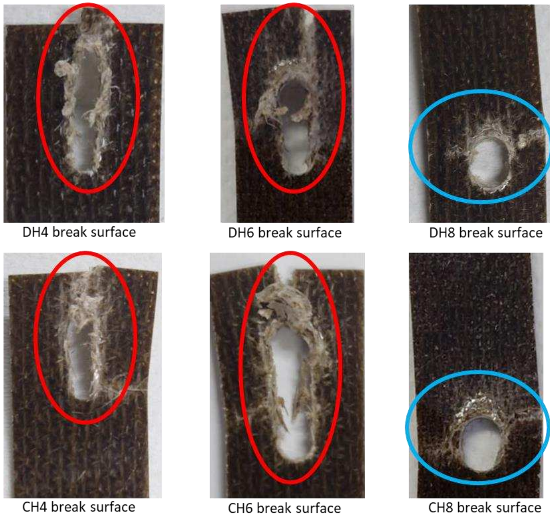
Figure 8. Fracture modes in bearing tests
