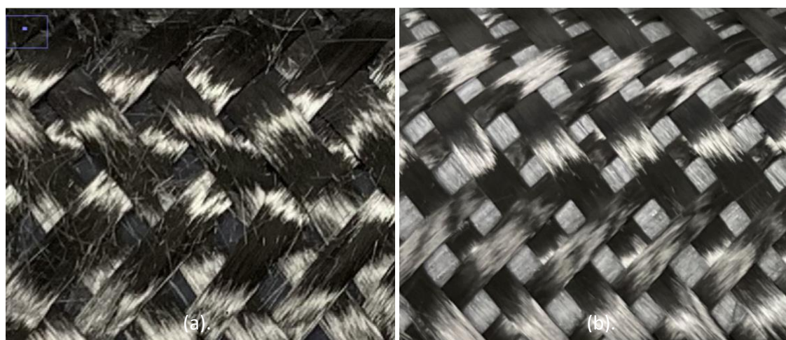
Figure 4 Images of the braided preforms (a) untwisted, (b) twisted
