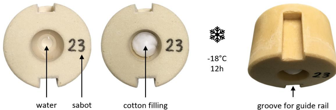
Figure 10. Freezing of sabot hailstone system before tests with 25mm artificial hailstones
