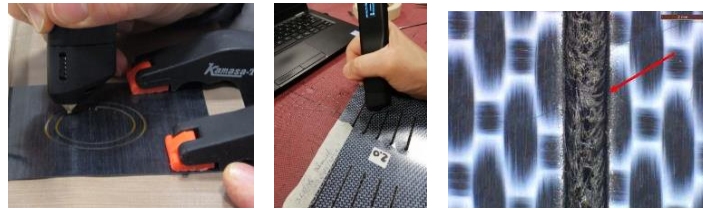
Figure 7. Deposition of the filler in the gaps by 3DPen and microscopic analysis before the CM
