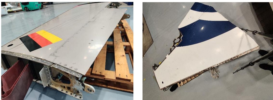
Figure 1. The two end-of-life vertical tail planes from which the carbon fibres were reclaimed and subsequently chopped for analysis
