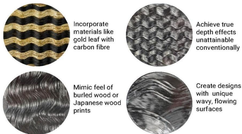
Figure 2. AFT offers options to create unique surface finishes by way of surface fiber layups that can even produce biomimetic looks. This feature is currently being used to produce structural, functional parts with unique surfaces in the motorsports and luxury consumer goods markets.
