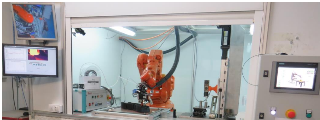
Figure 1. Robotic 3D printing cell developed.
