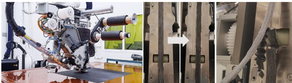
Figure 4: Picture of the AFP system used (left) and the processing of rCF-tapes with their challenges as homogeneity (middle) and wrinkling (right).
