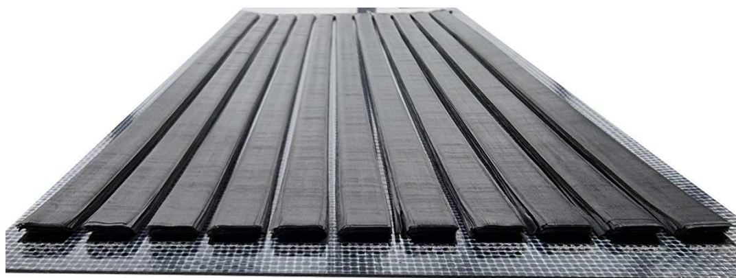
Figure 2. Nine test samples manufactured by laser tape placement with different permutations of tape and substrate temperature. The plain-woven CF/PEEK substrate and redundant samples at each end are also visible.
