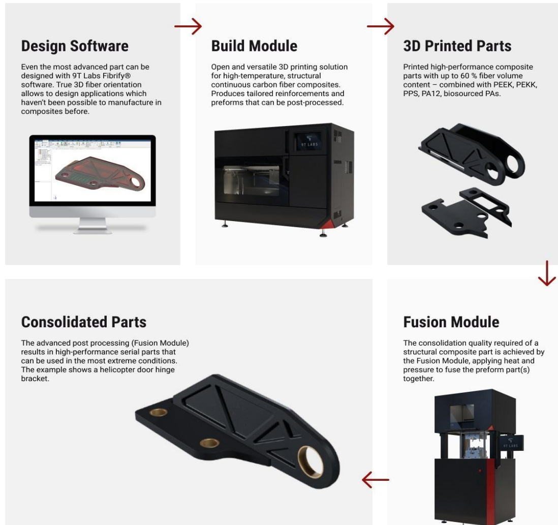
Figure 1. Additive fusion technology consists of advanced design software, a 3D printer that produces (near)-net-shape preforms, and a compact compression press equipped with matched metal dies in which preforms are heated, shaped, and consolidated.
