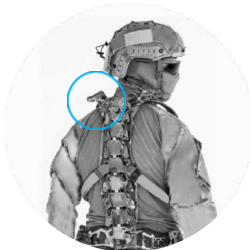
Figure 6: Benchmark exoskeleton winglet element produced in machined titanium.
