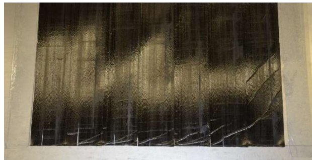
Figure 3: Wrinkles at the end of tracks caused by displacement of material
