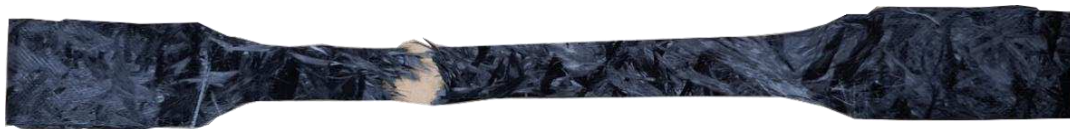
Figure 5: A sample Tensile test specimen after test
