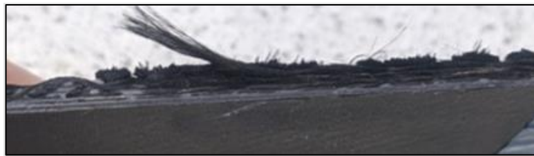
Figure 8. Cross section of a test coupon exhibiting clear interlaminar zone boundary
