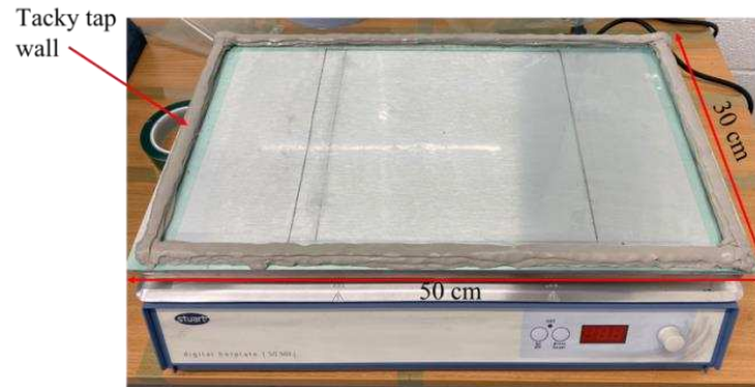
Figure 1. Hot-plate mould for curing epoxy-hardener system
