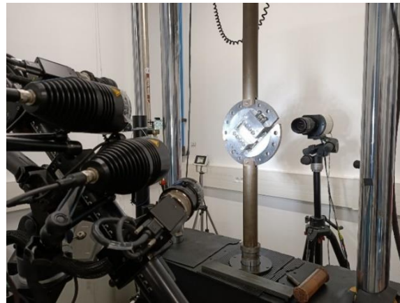
Figure 2: Arcan experimental set-up for fatigue tests
