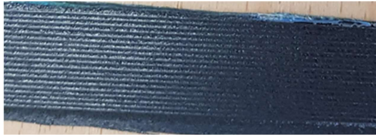
Figure 5. A cured thick ply prepreg sandwich: Skyflex K51 thin ply unidirectional carbon fibre, Skyflex K51 resin and Hyperflight 0.7mm diameter carbon fibre-epoxy pultruded rods
