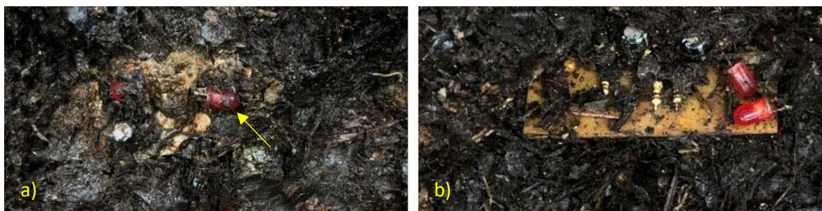
Figure 5. a) Fully degraded CNF substrate (an LED can be seen in the center of the image), b) well preserved PCB made of glass fiber reinforced epoxy.
