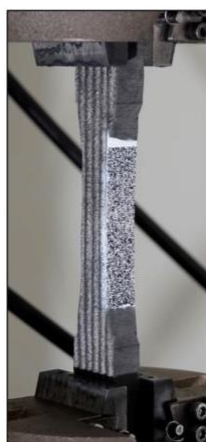
Figure 4 : ASTM D638-14 test setup
