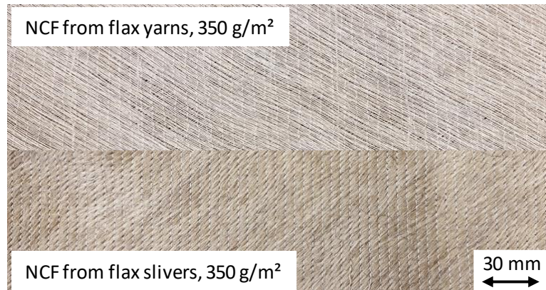
Figure 2. Comparison of NCF produced from flax yarns (top) and flax slivers (bottom)
