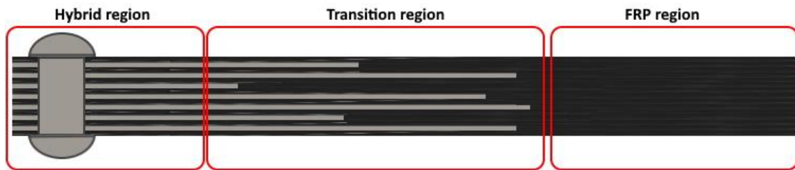
Figure 1 - Schematic representation of a locally hybridized mechanically fastened joint
