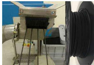
Figure 5. Filament extrusion and produced spool of filament
