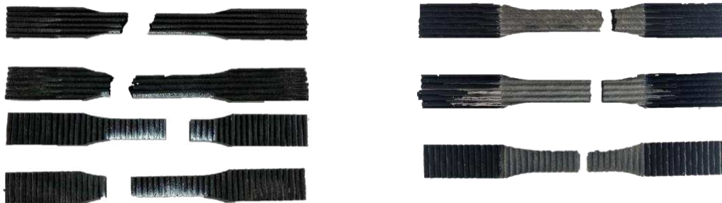
Figure 9: Tension testing – failed specimen images (left) PETG/CF & (right) PC/CF
