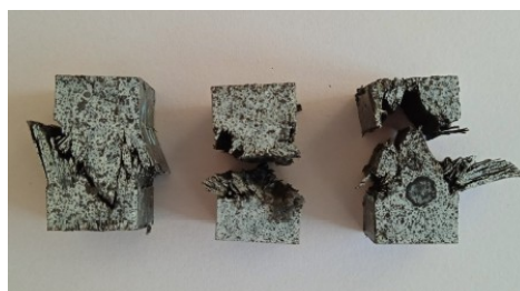
Figure 6. Failure modes in SHPB experiments
