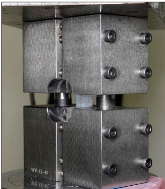
Figure 7 : ASTM D6641-14 CLC test setup
