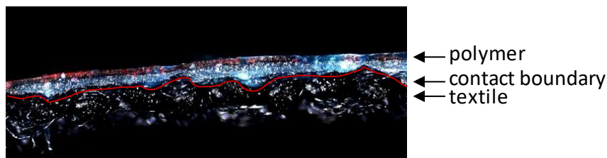
Figure 1 : Cross section of a polymer-textile composite
