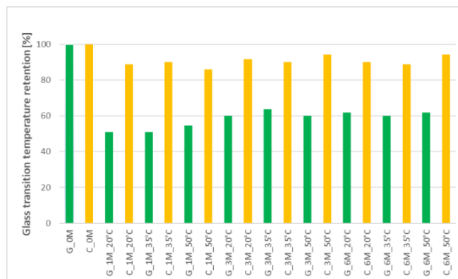
Figure 1: Retention of glass transition temperature for bio-based (GFRP_G) and petro-based (GFRP_C) GFRP composites during hygrothermal ageing
