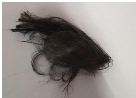
Figure 1 - Fluffy recycled carbon fibers.
