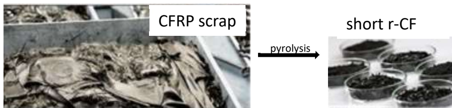
Figure 3. Short recycled carbon fibre (short r-CF)
