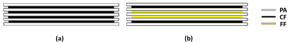
Figure 1: Manufacturing layup configurations: (a) non-hybrid carbon fiber composite (CCCC), (b) hybrid carbon-flax composite (CFFC).
