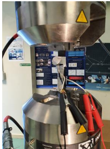
Figure 2. Lap Strap specimen during mechanical testing.
