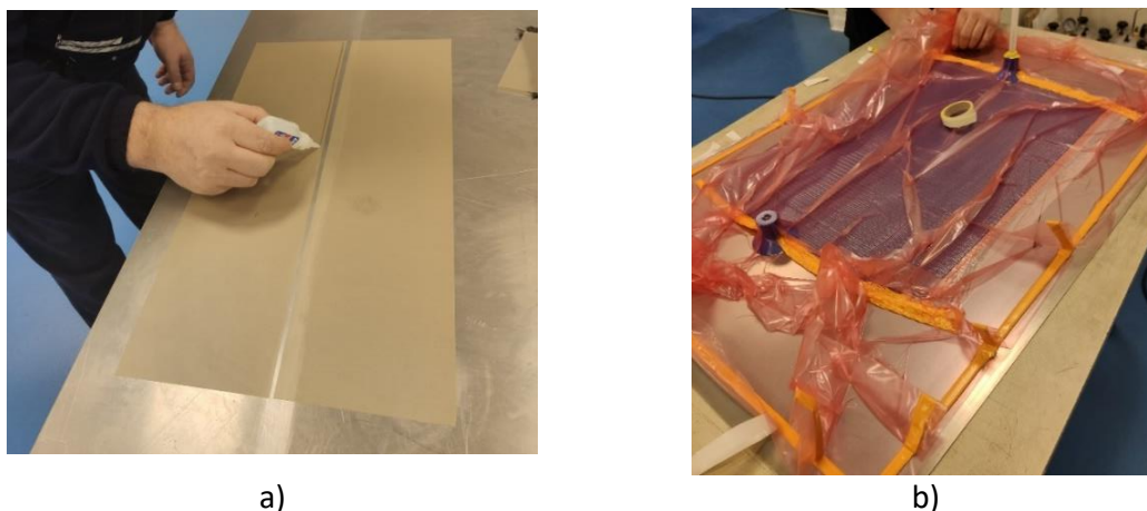
Figure 1. Manufacturing process of samples for welding tests
