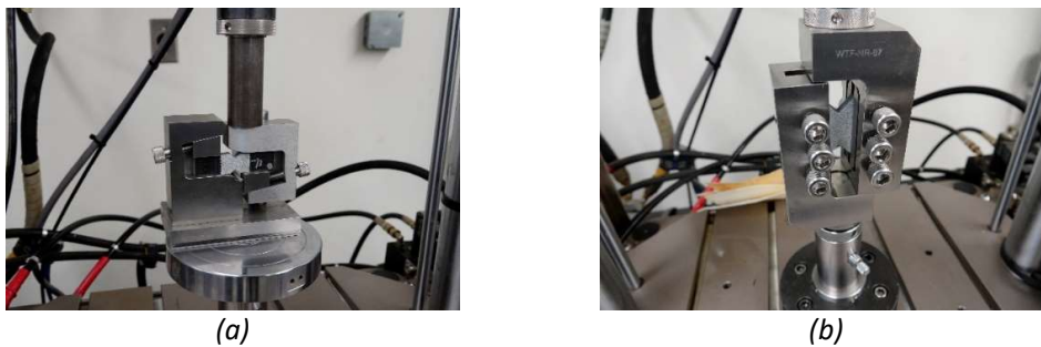
Figure 2. Test setup for (a) ASTM D5379 and (b) ASTM D7078.
