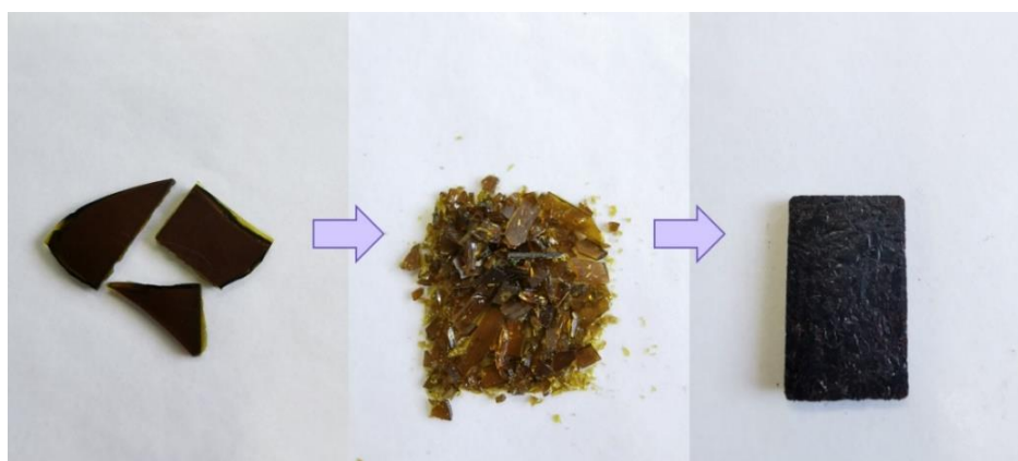
Figure 3: RTM6 vitrimer ( T_g > 210^\circ\text{C} ) reprocessed using a hot-press after grinding.
