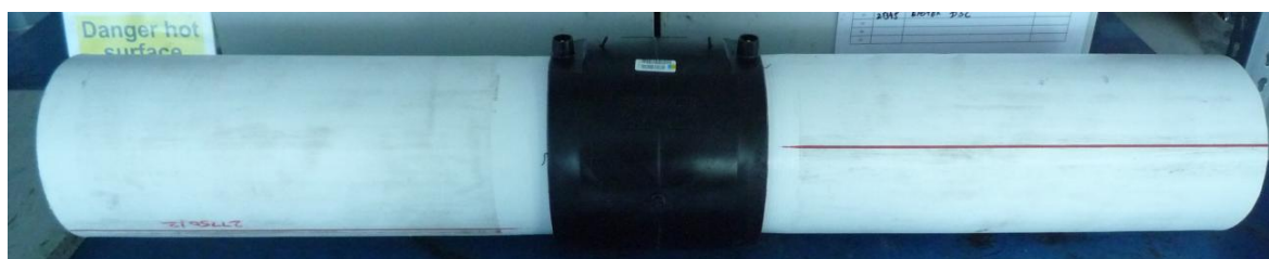
Fig. 4 One of three test samples – an electrofusion joint between two lengths of glass fibre reinforced polyethylene TCP
