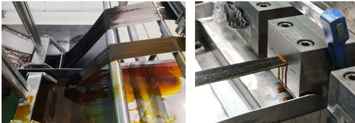
Figure 2. Pilot production of pultruded CFRP bio-laminates using the BUPE resin.
