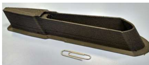
Figure 6. Flying part trial specimen printed to assess the process
