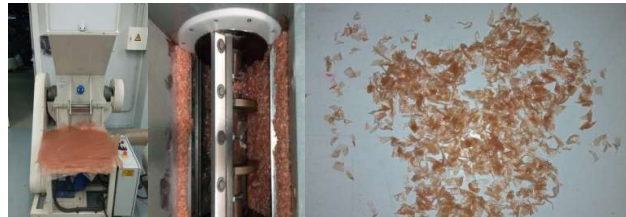
Figure 2. Vacuum bags shredding process
