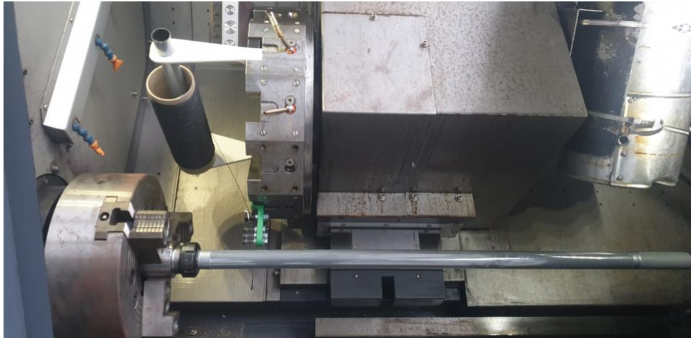
Figure 2: CNC modified for filament winding
