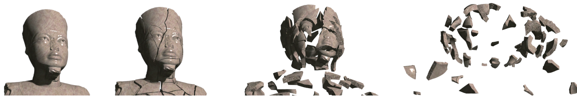
Figure 5.7: Brittle fracture of a hollow stone sculpture. Forces acting on the interior create stresses which cause the model to fracture and explode. Initial/final sampling: 4.3k/6.5k particles, 249k/310k surfels, 22s/frame.
