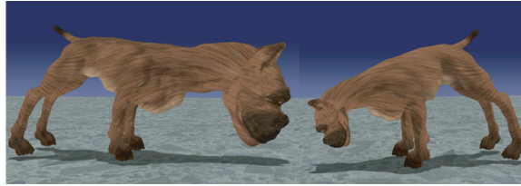
Figure 3.2: The pit bull with its inflated head (left) shows the artifact of linear FEM under large rotational deformations. The correct deformation is shown on the right [MG04]. Image courtesy of Matthias Müller, AGEIA/NovodeX.
