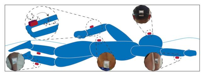
Figure 3.3 – IMU-based measurement setup. Six IMUs were attached to shanks, wrists, sacrum and head using waterproof tapes. During functional calibration, for each segment, the data will be transformed from sensor frame  $(\mathbf{x}\mathbf{y}\mathbf{z}_{\mathbf{s}})$  to anatomical frame  $(\mathbf{x}\mathbf{y}\mathbf{z}_{\mathbf{s}})$ .
