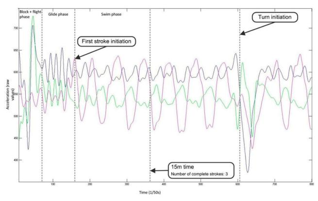
Figure 2.3 – Qualitative separation of swimming start on the acceleration signals from a back worn IMU with the aid of cameras. Adapted with permission from (Le Sage et al., 2012).
