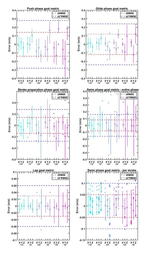
Figure 5.6 – Estimated goal metrics change with and without functional calibration along with the corresponding estimation RMSE. The rotation angle varies between  $10^{\circ}$  to  $30^{\circ}$  about each axis in both positive and negative directions.
