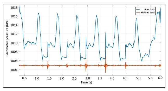
Figure 7.1 – Pressure profile of signal measured by the wrist barometer and its high pass component illustrating the water entering events.
