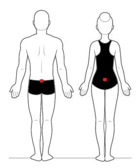
Figure 7.2 – Possible schematic for sensor integration into the swimming suit of swimmers (M/F)
