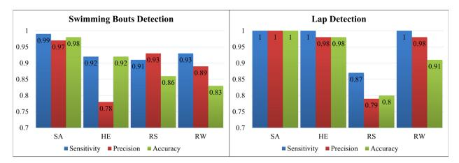
Figure 3.6 – Sensitivity, precision and accuracy achieved for swimming bouts and laps detection on all sensor positions (SA, HE, RS, RW)
