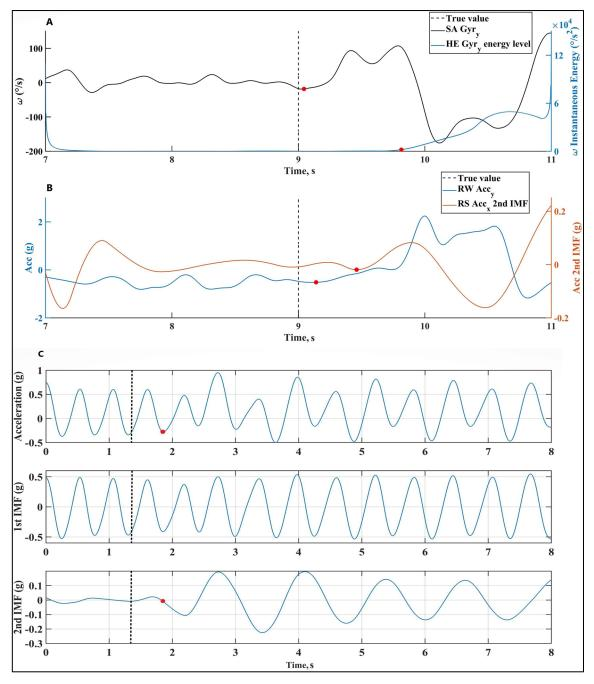
Figure 3.8 – An example of  $Swim_B$  event detection on all sensor positions. **(A)**  $Swim_B$  detection on SA and HE during front crawl, **(B)**  $Swim_B$  detection on RW and RS during front crawl, **(C)** an example of the process of using EMD technique for  $Swim_B$  detection during butterfly technique. It is shown that the second intrinsic mode function (IMF) separates the motion after  $Swim_B$ . The estimated values are represented on the corresponding signal with red dots.
