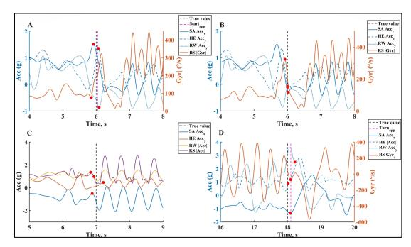
Figure 3.7 – An example of the swimming phases beginning event detection, (A)  $Push_B$ , (B)  $Glid_B$ , (C)  $StPr_B$ , (D)  $Turn_B$ , on all sensor positions during front crawl. The estimated values are represented on the corresponding signal with red dots and the true value is shown as a vertical dashed line.
