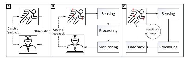
Figure 2.2 – Three types of technique analysis and feedback loops, based on coach involvement and measurement devices: **(A)** coach-based feedback, **(B)** coach-based feedback with technology equipment, and **(C)** autonomous feedback during technology-enhanced motor learning. Adapted from (Kos and Umek, 2018a).
