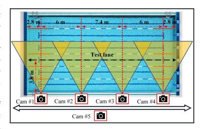
Figure 3.2 – Validation system including four cameras (Cam#1 - Cam#4) distributed along the pool in the same depth (0.5 m) underwater and one camera (Cam#5) moving with swimmer in land to capture the events over water
