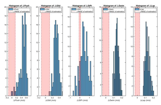
Figure 5.3 – Histograms of changes in the five IMU goal metrics ( $\Delta Push$ ,  $\Delta Glid$ ,  $\Delta StPr$ ,  $\Delta Swim$ , and  $\Delta Lap$ ) for the comparisons with meaningful progress. The estimation *RMSE* range of each goal metric is displayed with red dashed lines.
