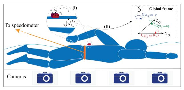
Figure 4.1 – Measurement setup, including one IMU attached to the sacrum, four cameras to capture the whole lap and tethered speedometer to record swimmer's displacement and velocity. IMU data is transferred from sensor frame (x,y,z)s, first to anatomical frame (x,y,z)A using functional calibration (I), and then to the global frame (X,Y,Z)G using the gradient-descend based optimization algorithm (II). The global axes of acceleration, angular velocity and angles are displayed in the figure.
