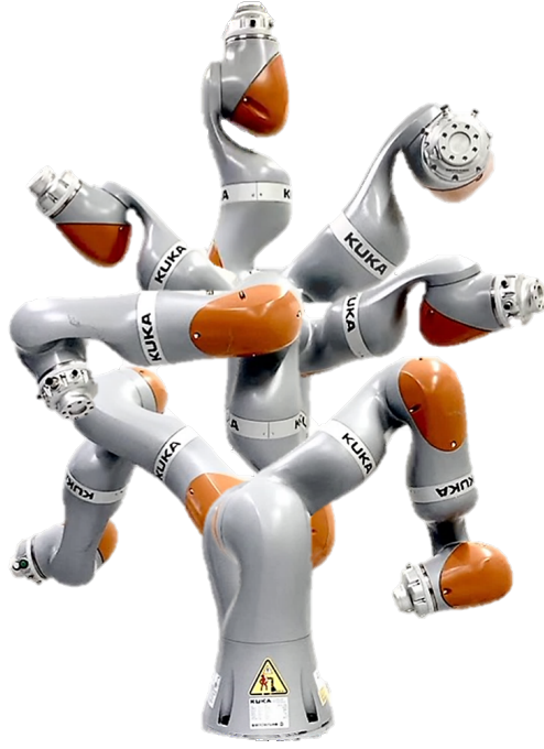
Figure 1.4: Different examples of robot configuration during exploration of the KUKA LBR iiwa 14 joint space when using our configuration exploration approach.
