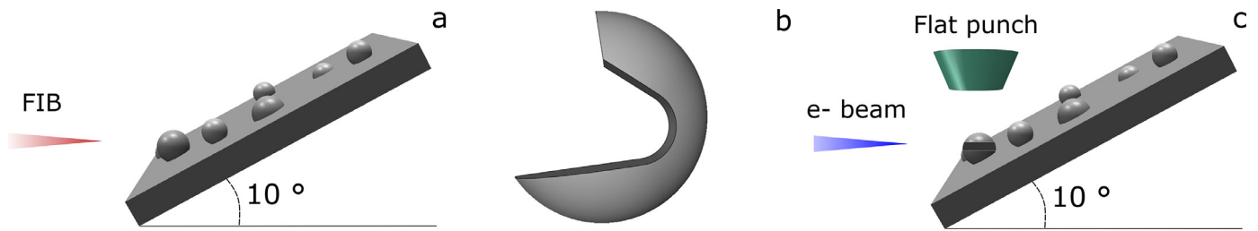
Fig. 2. Schematics of (a) the positioning of samples for FIB milling; (b) the notch geometry used for the testing of spherical inclusions (viewed along the direction of the ion or electron beams); (c) subsequent positioning of the sample for in-situ testing in the SEM.
