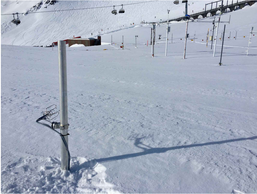
Figure 2.10: The sonic anemometer installed in the field
