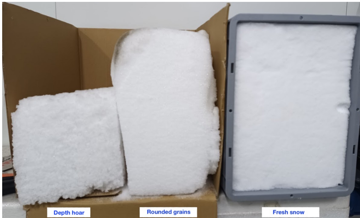
Figure 4.24: Picture of three different snow types scanned (photo: Benjamin Walter)
