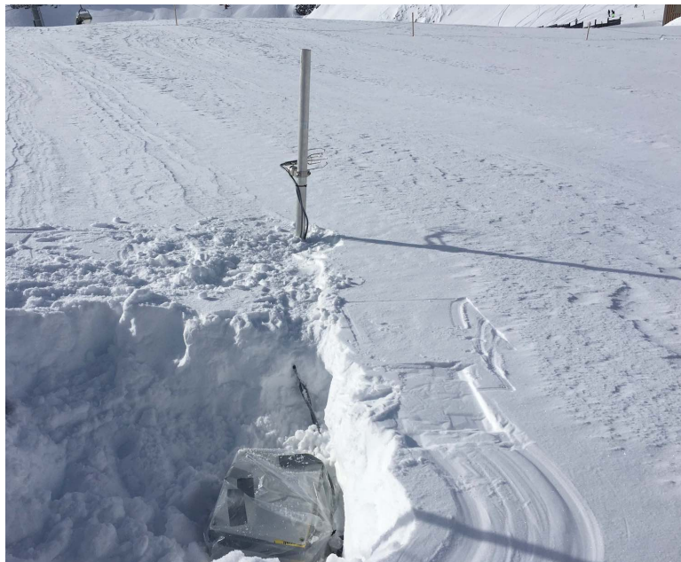
Figure A.8: Installation of the sonic anemometer, the waterproof box contain the converter.
