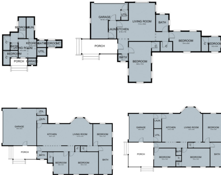
Floor plan optimization going from 200, 2 000, 20 000 and 100 000 iterations
