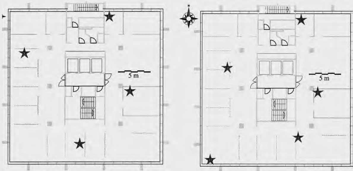
Figure 2: Location of TinyTak monitoring thermometers. Left: second floor, right: tenth floor
