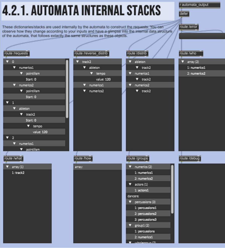
Figure 25 Capture of the automaton debug and convenience panels representing each object (stack) internally used by the automaton
