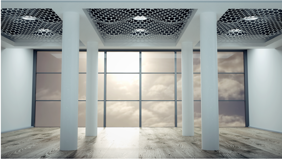
Figure 7: Interior decorative cladding. This hanging structure has been optimized to align with the boundary constraints imposed by the ambient space. The designer controls the shape by interactively modifying scale factors.
