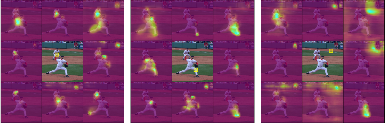
Figure 4: Attention maps of the relationship head’s Transformer. For a given reference point (yellow box), the attention maps from all heads of the last self-attention layer are shown. Order of heads is arbitrary. Attention heads are able to attend to the surroundings of the cell as well as far-away objects.
