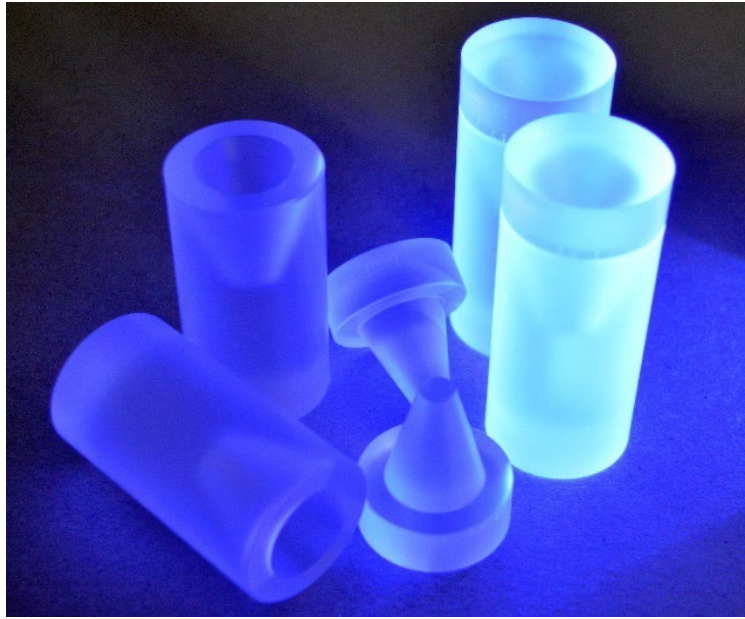
Fig. 4.49: Plastic scintillator vials illuminated by UV light to stimulate the emission of scintillation light (taken from [214]).
