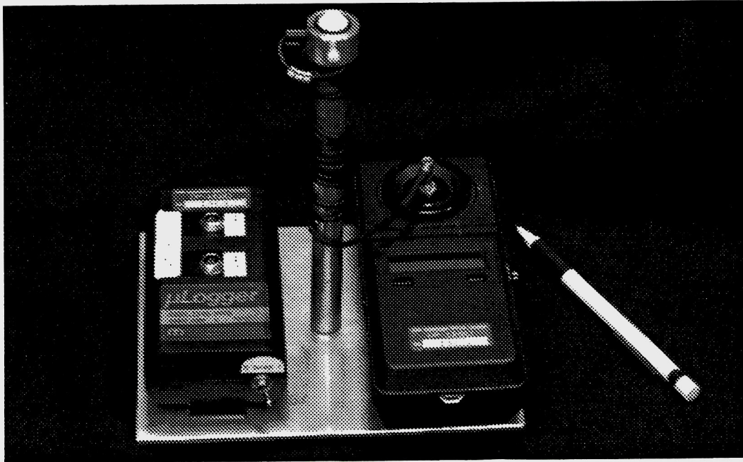
Figure 2.47: View of the illuminance sensor and its holder, placed on a desk.
