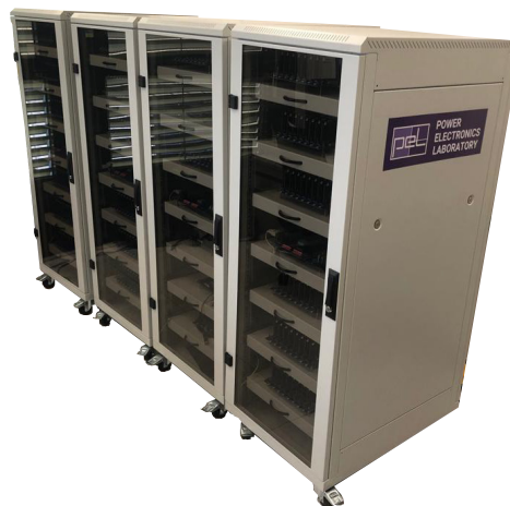
▲ Digital Twins - Four RT-HIL systems allowing for various topological reconfigurations
