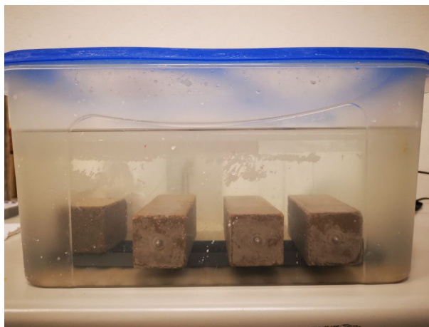
Fig. 3-2 Full immersion test container with 4 mortar prisms.
