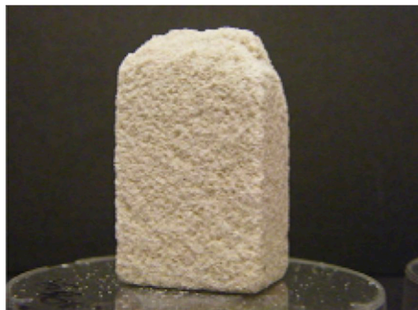
Fig. 2-13 Granular disintegration of the salt-contaminated sandstone [30].
