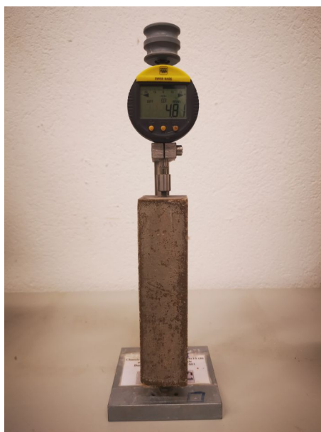
Fig. 3-5 The expansion measurement of the mortar prism in the submerge test.
