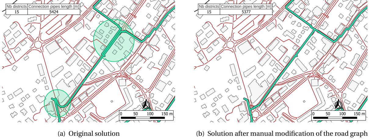
Figure 2.28: Improvement of the solution by manually modifying the road graph. The red lines are the graph imported from the library and the blue line the DHN pathway solution. Lines of the graph are deleted in (b) to avoid inconsistency.
