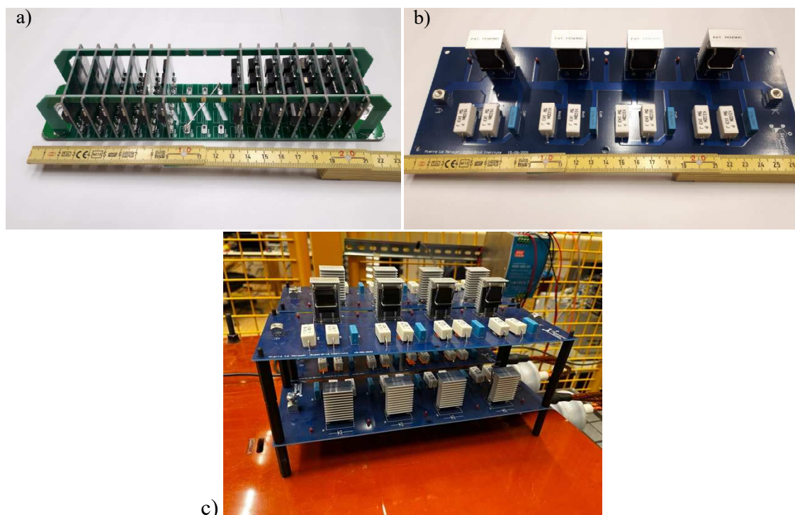
Fig. 3: a) An example of commercially available high voltage diode assembly, intended for forced air or oil cooling; b) Diode assembly composed of four series connected diodes, designed for natural convection cooling c) Full-bridge rectifier composed of 4 diode assemblies.
