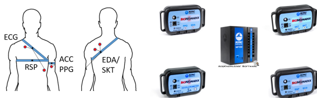
Fig. 7: Sketch of the BIOPAC [29] sensors positioning (left) during the experiment and the sensors themselves (right)
