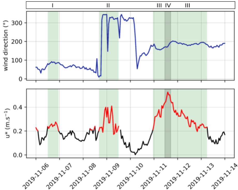
Figure 3. Time series for wind direction (top) and surface friction velocity at 2 m (bottom) measured in the period between the successive TLS measurements. The values displayed are an average of measurements taken at 2, 6 and 10 m height. The green-colored areas (I to III) correspond to the time periods for which snow movement was assumed to occur. The darker area (IV) shows the time span during which precipitation was measured by the radar. Source: Cox et al. (2021).
