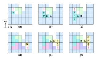
Fig. 9. (Top) Construct  $P_2$  in the configuration  $C_{\text{prim}}$  in Figure 7(b). (Bottom) Construct  $P_5$  in the configuration  $C_{\text{prim}}$  in Figure 7(e). (a&d) Select a moving direction  $d_i$  and a seed voxel S. (b&e) Select a pair of blockee and blocking voxels (marked as  $B_e$  and  $B_i$  respectively) and connect the seed voxel S with the blockee voxel  $B_e$  using a shortest path (voxels on the path are marked as P). (c&f) Expand the puzzle piece.
