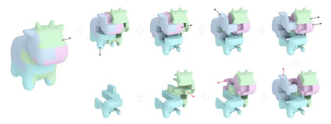
Fig. 1. A 4-piece level-6 interlocking puzzle designed by our approach that requires 6 moves to take out the first piece (in blue color). Each sub-figure shows a configuration of the puzzle pieces in the disassembly plan, where arrows indicate the translational direction to move (in black) or remove (in red) a subassembly to reach the next configuration. Note that the two black arrows in the top right subfigure indicate a single move of a subassembly with two parts.
