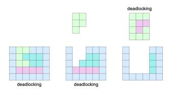
Fig. 6. Three cases of deadlocking puzzles. From left to right, the whole puzzle, the puzzle after removing the green piece, and the removed subassembly, are deadlocking.
