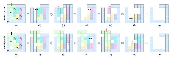
Fig. 2. Comparing a level-1 interlocking puzzle (top) and a level-5 interlocking puzzle (bottom). (Top) The puzzle requires one move to take out the first piece ( $P_1$ ); each of the remaining puzzle pieces requires two moves to be taken out. (Bottom) The puzzle requires five moves to take out the first piece ( $P_1$ ), where the 2nd move translates two puzzle pieces ( $P_4$  and  $P_5$ ) together; after taking out  $P_1$ , each of the remaining puzzle pieces can be taken out easily.
