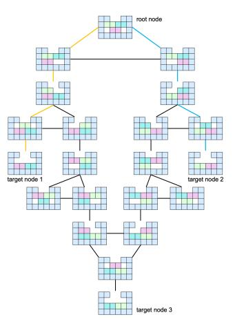
Fig. 5. The kernel disassembly graph of a 4-piece level-4 interlocking puzzle. The graph has three target nodes, and the exact level (i.e., 4) of the puzzle is defined by the shortest path from the root node to the target node 1 or 2 (the path is colored in orange or cyan respectively).
