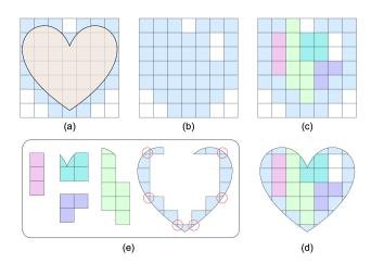
Fig. 10. (a) Voxelizing a given smooth shape. (b) Taking the voxelized shape (with two hole voxels) as an input, we generate a (c) 5-piece level-2 interlocking puzzle by using our design approach in Section 5. (d) A puzzle with smooth appearance is obtained by performing CSG intersection between each voxelized puzzle piece in (c) and the input shape in (a). (e) However, the generated puzzle pieces are possible to be structurally weak for fabrication and playing (see red circles).
