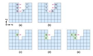
Fig. 8. Constructing the first puzzle piece  $P_1$ . (a&b) Candidates of seed voxels (marked as *S*) for  $d_1 = +x$  and  $d_1 = -x$  respectively, where there should exist voxels (marked as *T*) that stop  $P_1$ 's movement along  $d_1$ . (c) Choose a seed voxel for the first puzzle piece and (d&e) incrementally expand the piece by adding voxels (marked as *E*) one by one.
