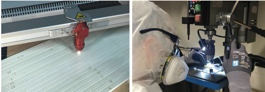
Figure 5: Etching and drilling the GFRP rods.
