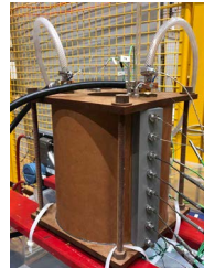
▲ Oil vessel instrumented with thermocouples.
