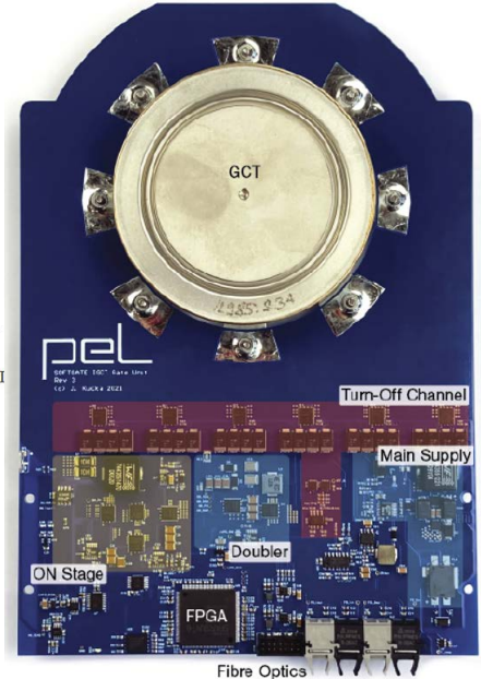
▲ Realized SOFTGATE gate unit [39]
