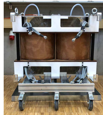
▲ 1 MW prototype of the 2-vessel MFT structure.
