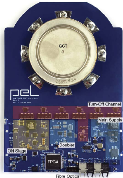
▲ Realized SOFTGATE gate unit
