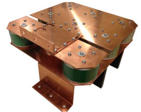
▲ (left) Custom made amorphous alloy core magnetizing inductor; (middle) Configurable array of eight air core resonant inductors; (right) Reconfigurable resonant capacitor bank
