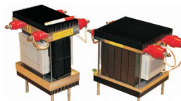
CHALMERS: 50kW, 5kHz
