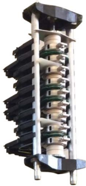
▲ (left) ABB ACS1000 water cooled 3L-NPC IGCT stack (DUT); (middle) Custom-built diodes stack; (right) De-ionised water cooling unit
