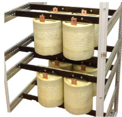
▲ (left) Custom made amorphous alloy core magnetizing inductor; (middle) Configurable array of eight air core resonant inductors; (right) Reconfigurable resonant capacitor bank
