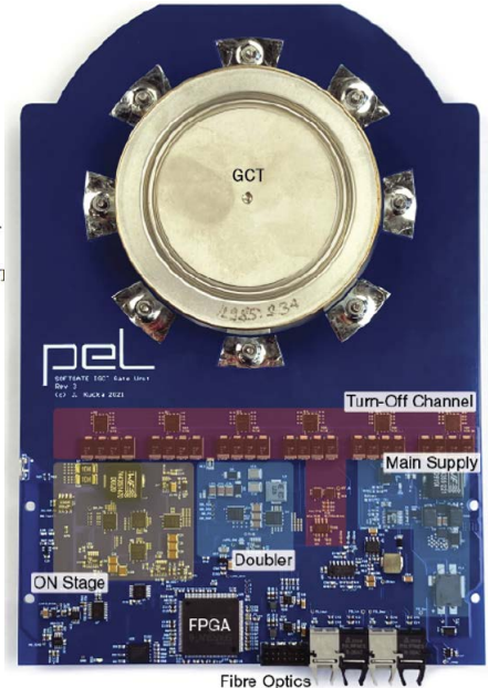
▲ Realized SOFTGATE gate unit
