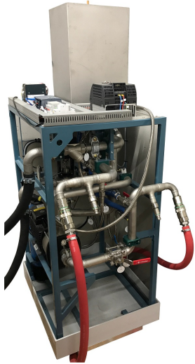
▲ De-ionised water cooling unit - limited temperature control.
